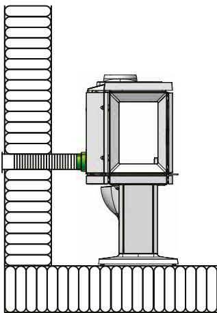
Fig. 3d Indirectly through an outside wall
