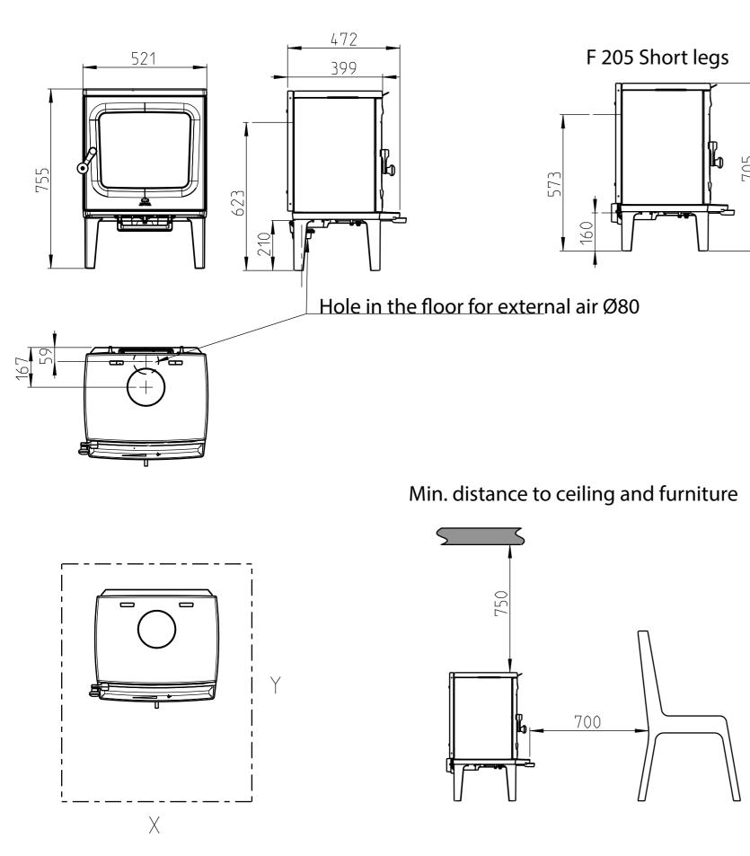
Min. measurments floor plate X/Y = According to national laws and regulations Min. distance to combustible wall
